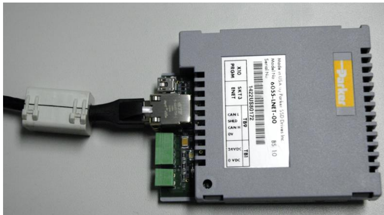
6055-LNET-00 TECHBOX with FERRITE CORE Installed
